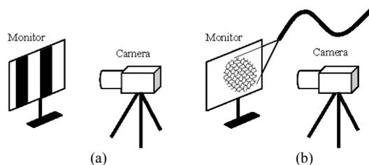
Figure 7. Projector calibration:
