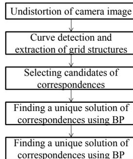
Figure 5. Algorithm of 3-D shape reconstruction.
