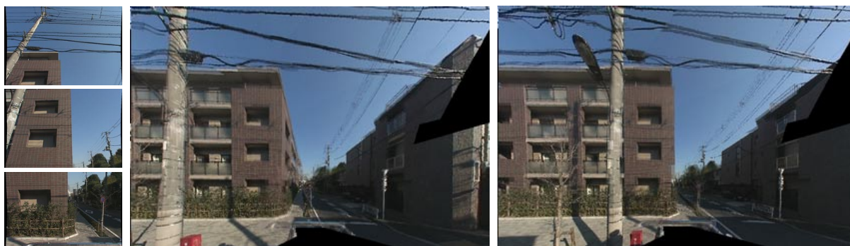
Figure 10: Result of stitching 9 images taken by omni-directional camera configured as Fig.2-(b). Because of the spatio-temporal synchronization technique, there are no distortions on either the electric pole and the buildings.
