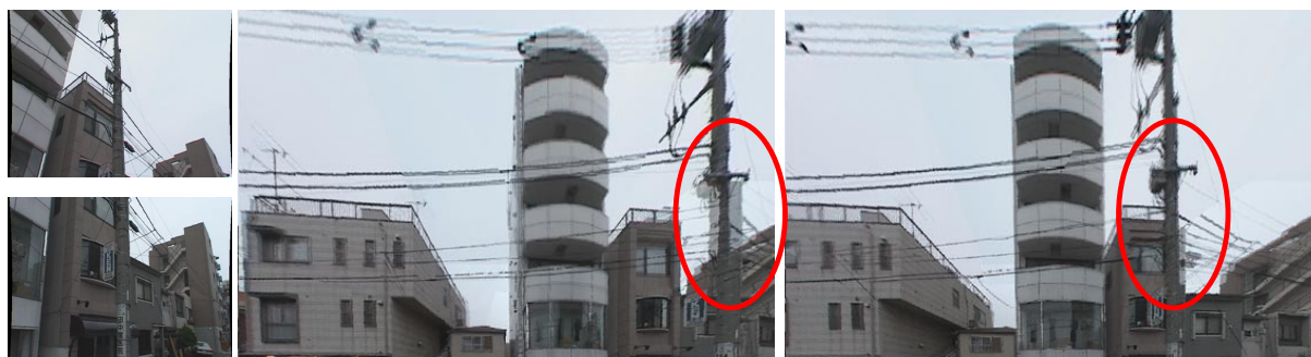
Figure 9: Another result of stitching 6 images taken by omni-directional camera configured as Fig.2-(c). Note that the depth of the buildings and the electric pole is largely different, therefore, distortion occurs in fused image.
